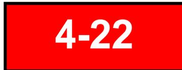
2. **Instrument Landing System (ILS) Critical Area Signs** – White letters on a red background. These signs indicate the edge of the ILS and may not be passed if told to “hold short” at the ILS by ATCT.
